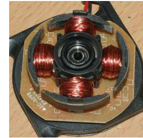
Brushless DC (actually a pulsed AC motor)
